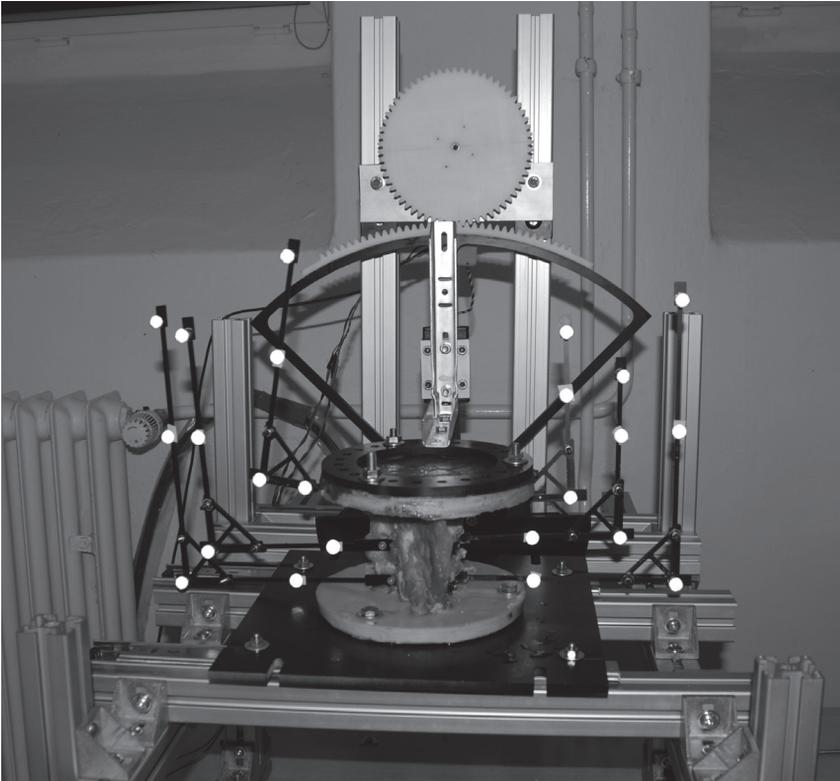
**Figure 3.** L5–L3 segments of porcine spine fixed into testing device. 8 reflex markers in two consoles was attached on each vertebra, one console with four markers onto procesus spinosus and second on ventral shape of vertebral body.
