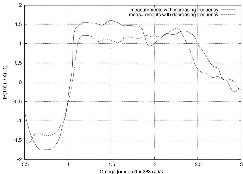
**Figure 4.** The transmission of the wave between two segments (Th9 and L1) during two measurements going one right after the first one. The x axis are the multiples of the resonant frequency and the y axis is the phase shift between the two measured segments. The phase shift around resonant frequency (25 Hz) is close to zero.
