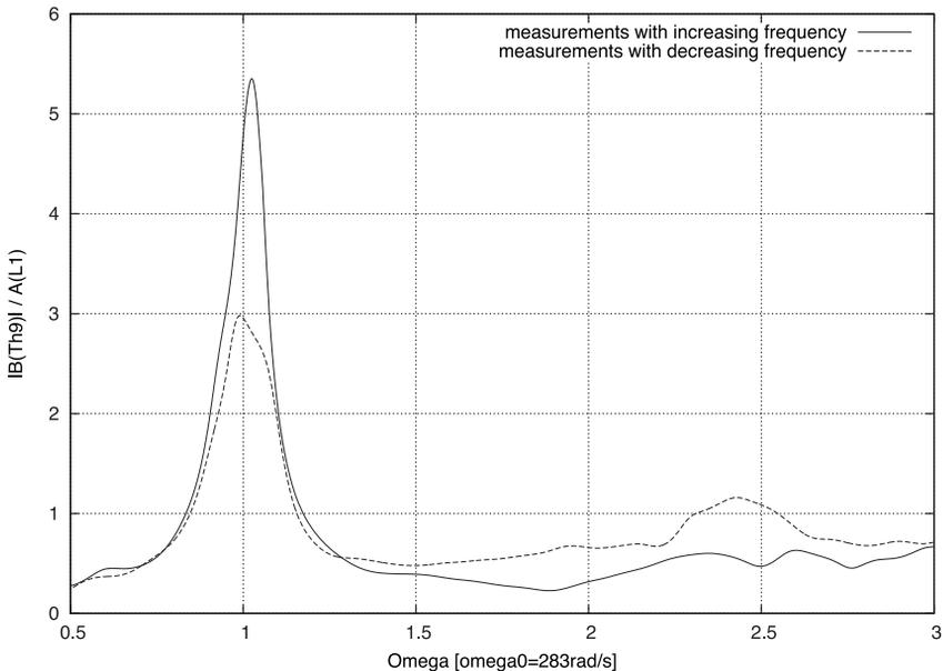
**Figure 3.** The transmission of the wave between two segments (Th9 and L1) during two measurements going one right after the first one – measurement with increasing and decreasing frequency. The x axis are multiple of the resonance frequency, 1 correspond to 25 Hz. The y axis is the ratio of output and input amplitude.
