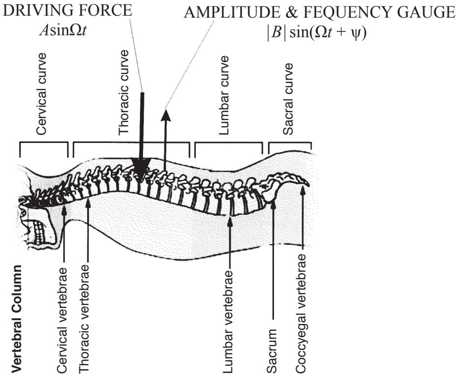
**Figure 1.** On the figure is the schema of measurement where  $A$  is amplitude of driving force,  $\Omega$  is momentaneous driving frequency,  $B$  is the amplitude of the answer,  $\psi$  is phase shift. The  $A \sin \Omega t$  is the input and the  $|B| \sin(\Omega t + \psi)$  is an output of the measurement.
