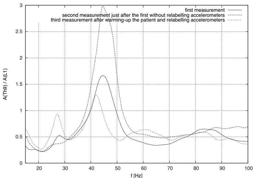
**Figure 5.** The ratio of amplitudes between the segments Th9 and L1 during the three measurements going in the row. The highest amplitude is when the person was relaxed and the damping was lowest, the lowest amplitude is when the person had some physical activity and the damping was highest.
