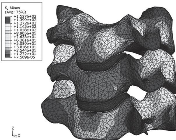
**Figure 10.** Segmentation of the 3D model into a finite number of elements allows to calculate the stress-strain characteristics in each element (<http://www.biomechanics.cz>, 2012)
