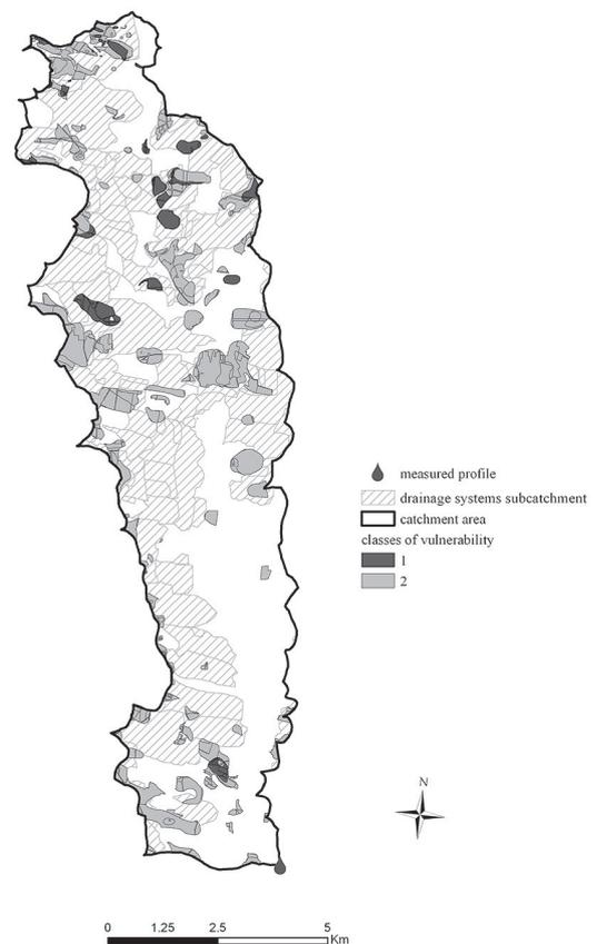
**Fig. 5** Drainage systems subcatchment (Bilinský brook)
