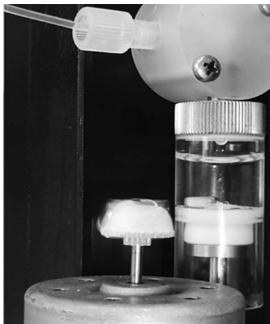
Fig. 1. In-syringe single-drop head-space microextraction with visible drop of reagent placed in the syringe inlet with applied vacuum.
