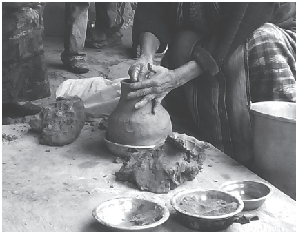
Figure 19. Rolling process, modeling of the neck and lip of a pitcher, San Mateo Ixtatán, Huehuetenango, Guatemala. Photo: Julio Hernández.
