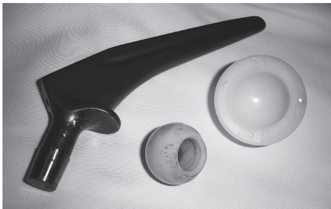
Fig. 3: A titanium hip prosthesis, with a ceramic head and polyethylene acetabular cup 13
