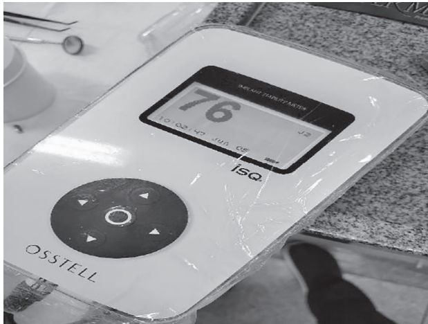
Figure 2: Implant stability quotient value provided by the Osstell device. 76 implant stability.
