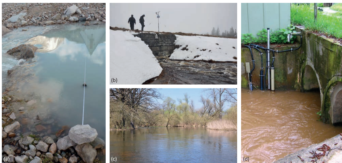
Fig. 3 Variability of physical properties of gauging stations. (a) Outlet from the Adygine lake. Water drains away via a stable bedrock ridge (riegel), (b) Gauging station of the Rokytka River at the time of maximum water level during the flood situation on December 1, 2015, (c) Lužnice gauging station site at the time of maximum measured water level, (d) Gauging station of the Mladotický Creek during period of increased water level.
