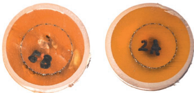
Fig. 2 Layer integrity of the nitinol wire, silicone coating and resin after waterjet cutting.
