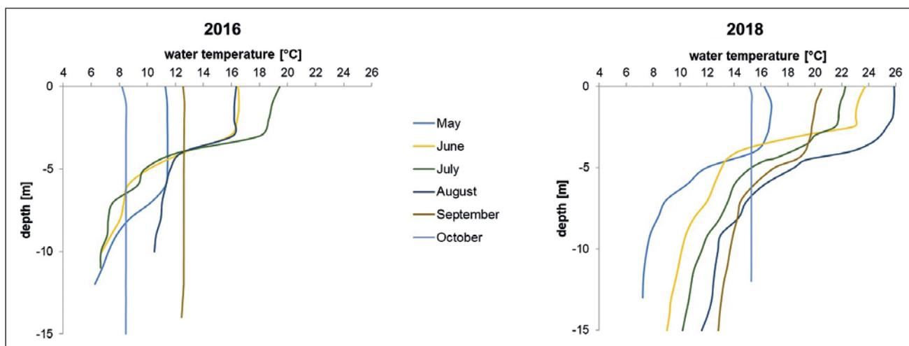
**Fig. 3** Thermal stratification – vertical profiles at S3 (2016, 2018).
