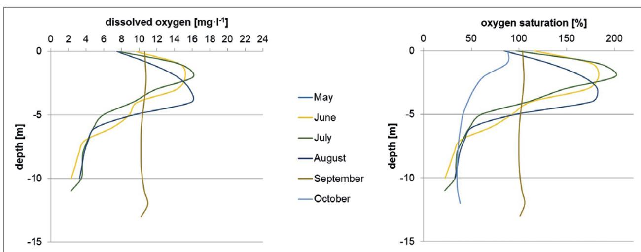
Fig. 5 Stratification of dissolved oxygen and oxygen saturation: vertical profiles at S4 in 2016.
