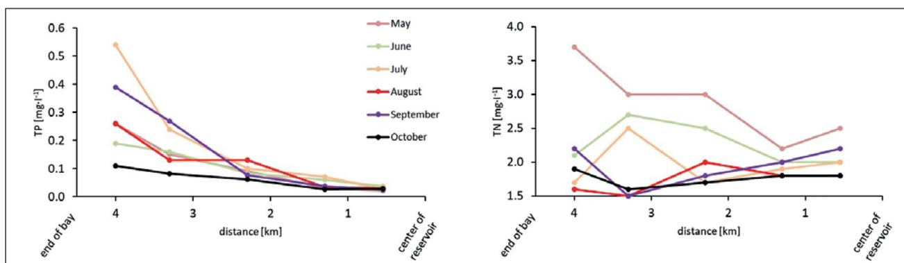
Fig. 6 Longitudinal profiles of TP and TN concentrations along Mastník bay in 2018 (mixed samples).
