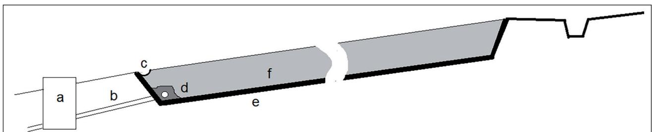
**Fig. 3** Scheme of the individual catchment transection: a) measurement shaft for subsurface runoff measurement (see Fig. 4 for details), b) pipe bringing subsurface runoff from drainage system, c) surface runoff collecting ditch, d) drainage, e) clay sealing, f) backfill.
