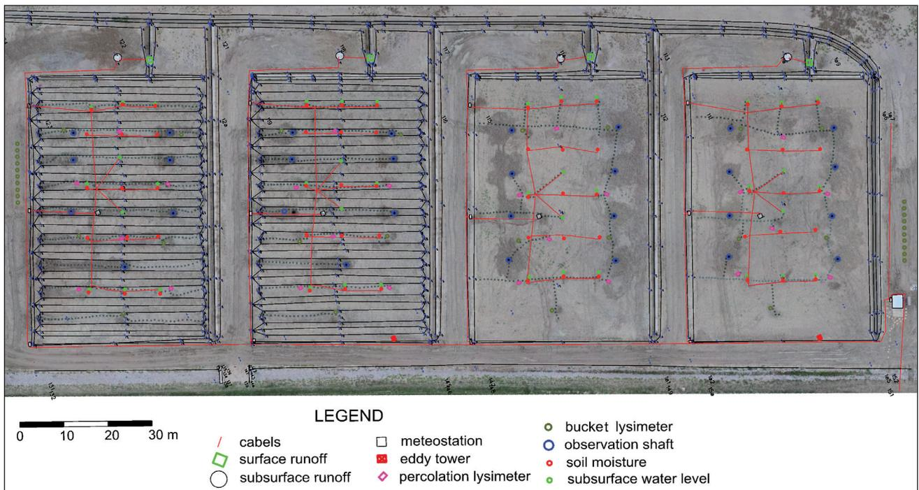
**Fig. 2** Aerial photo of whole catchment array and location of instrumentation in one of the catchments.
