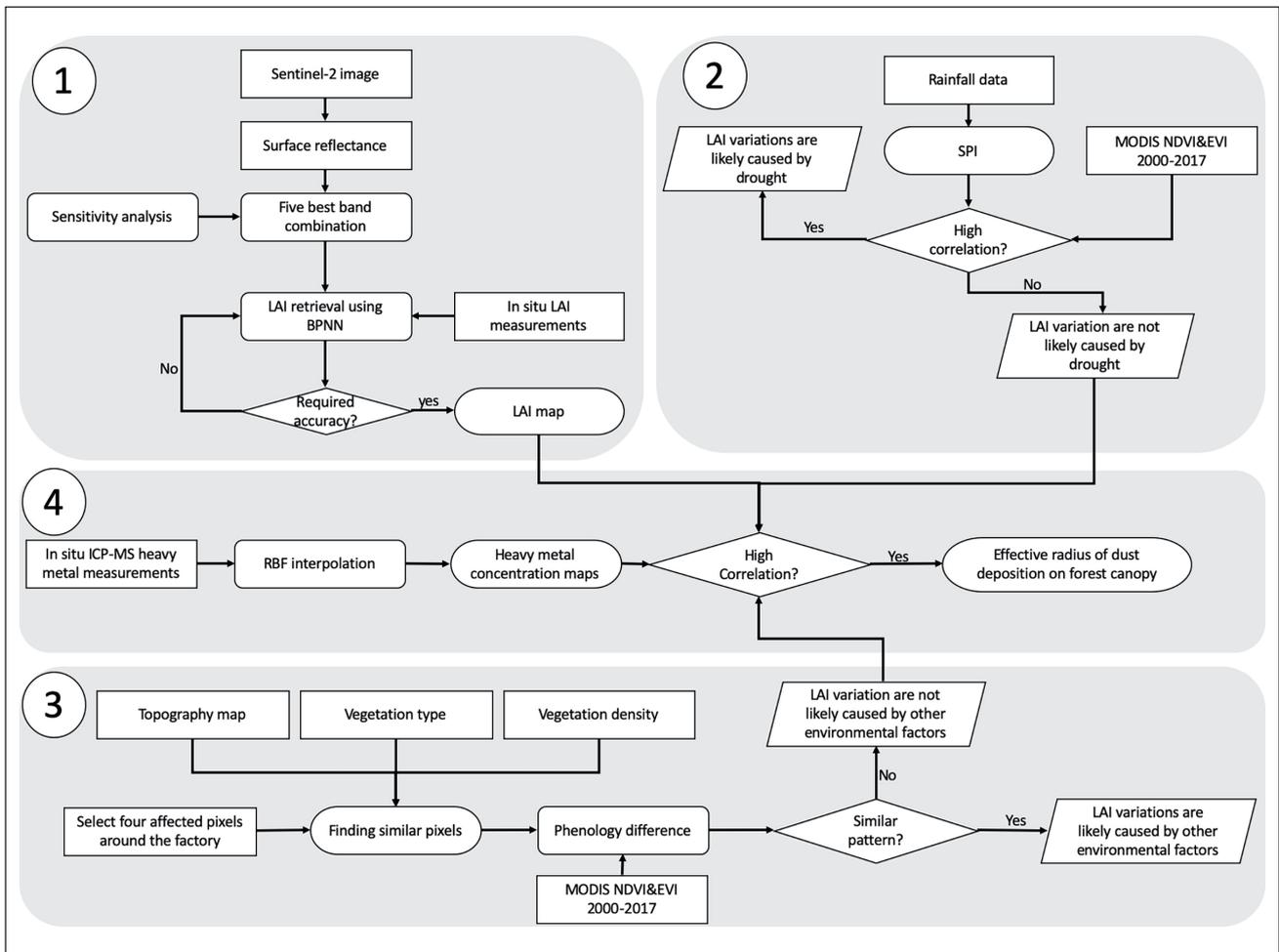
**Fig. 2** Flowchart of the methodology. LAI retrieval from Sentinel-2 image of September 22, 2017 (1); was used to check whether variations in LAI were caused by drought (2); or other environmental factors (3); which determine the effective radius of the deposition of dust on the canopy of the forest (4).
