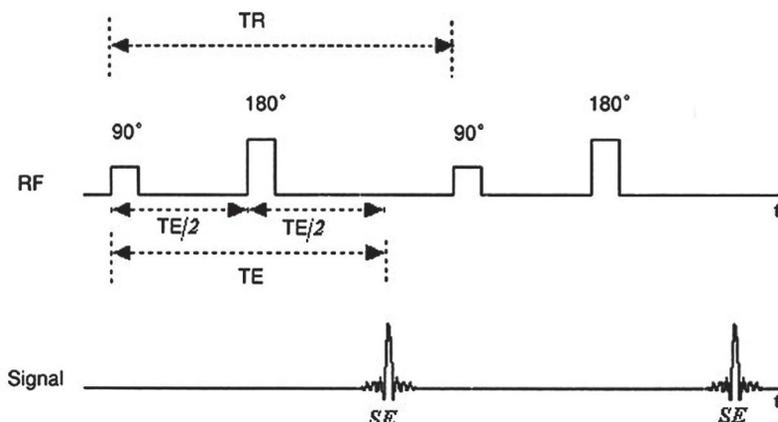
**Figure 1.** SE sequence consisting of 90° pulse and the subsequent 180° pulse. Figure edited from Fieremans (2009) and subsequently adapted
