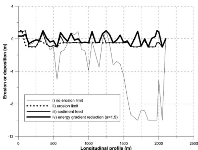
**Fig. 4** Modelled changes in the longitudinal profile due to erosion or deposition during the 5/2010 flood in Malá Ráztoka stream.
