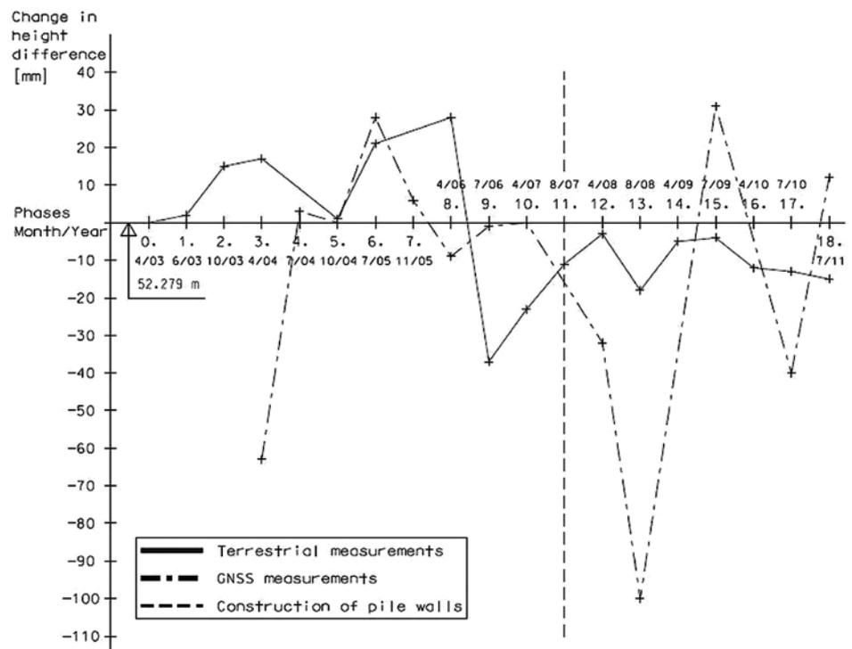
**Fig. 9** Changes in height difference between Rab01–Rab02 points.
