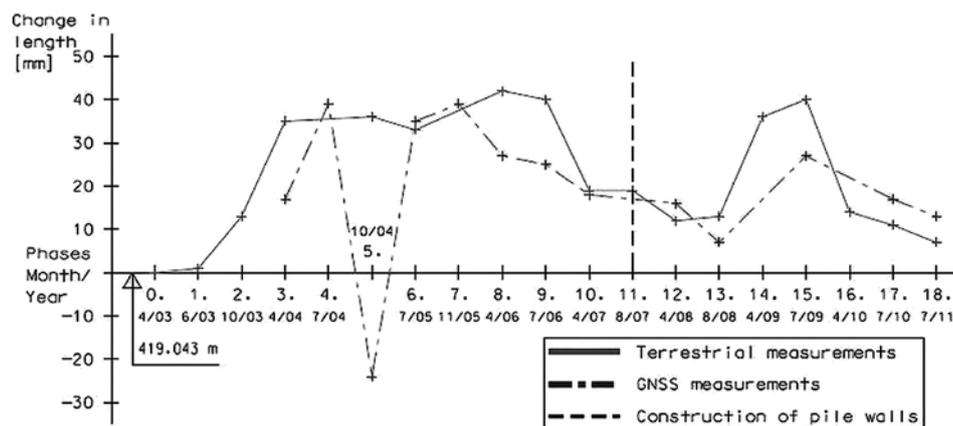
Fig. 7 Changes in length between Rab01–Rab03 points. Source: Rytíř 2012, Riegerová 2012
