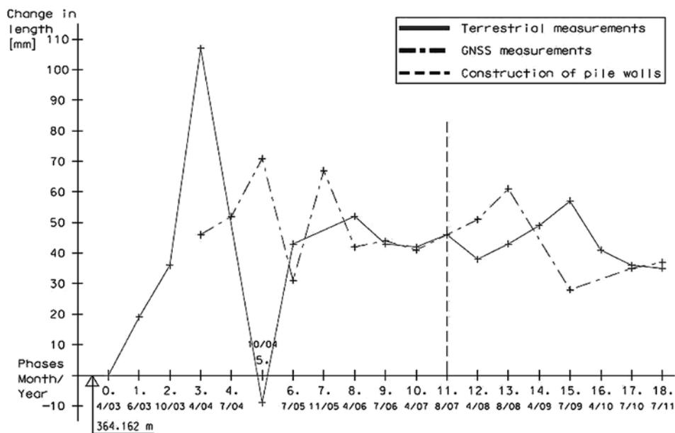
Fig. 6 Changes in length between Rab01–Rab02 points. Source: Rytíř 2012, Riegerová 2012
