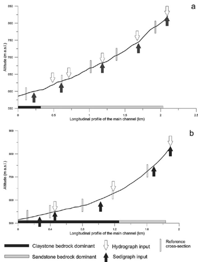
**Fig. 2** Schematic longitudinal profiles of Malá Ráztočka (a) and Velký Škaredý potok (b) used in simulations with indicated locations of inputs of water and sediments during a flood event.
