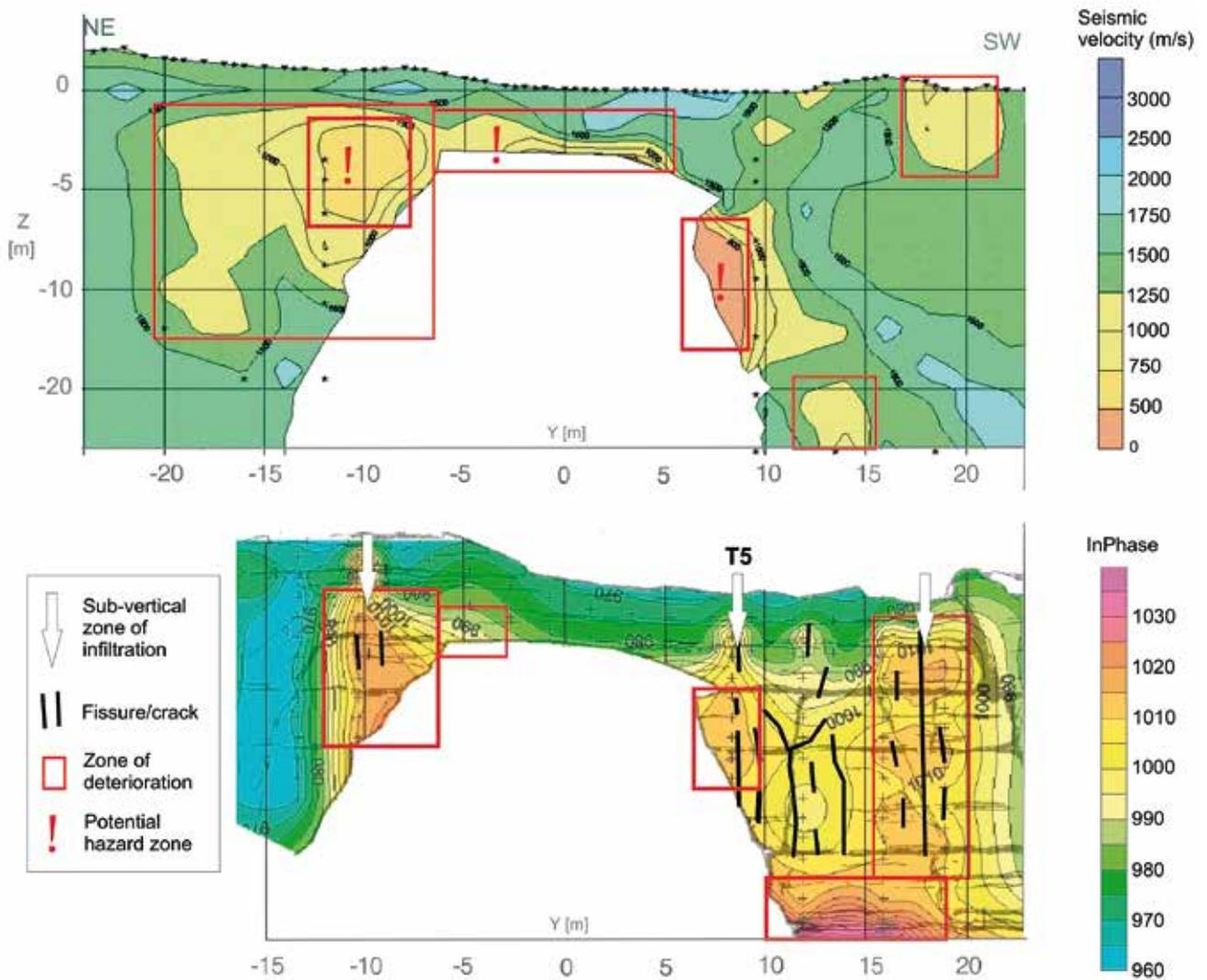
**Fig. IV** Map of seismic velocities in the western wall of the rock arch, identified by the method of seismic tomography (above), where red to yellow zones indicate the most weakened parts of the rock arch, correspond with Inphase profile (at depths of 3–4 m depth behind the rock wall) as a results of dipole electromagnetic profiling/DEMP (below) from which material changes in the rock (represented by violet/orange colour) can be inferred.
