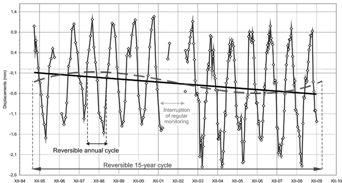
**Fig. 5** Graph of relative movements – data from manual measurements: Displacements at site PB 5 (average amplitude for whole monitored period amounts to 2.81 mm), with the annual and 15 year interspersed reversible cycle. Long-term irreversible trend of deformation is represented by the very slow closing of the measured crack (the black linear connecting line of trend more than 0.5 mm/15 years).
