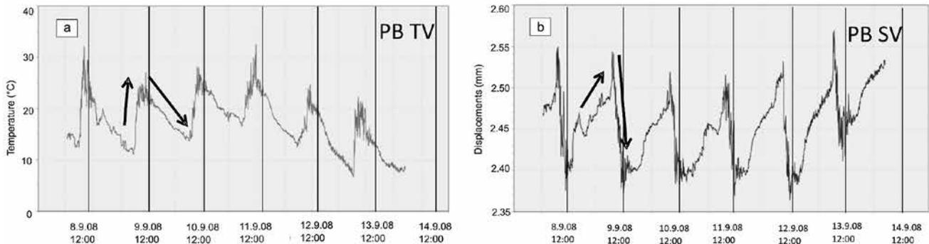
**Fig. 6 a)** Daily changes of temperature (a) and daily quasi-cycles of deformation (b) of the rock arch beam (example of an automatic monitoring data, from the sunny period 2008, site PB V on the east).
