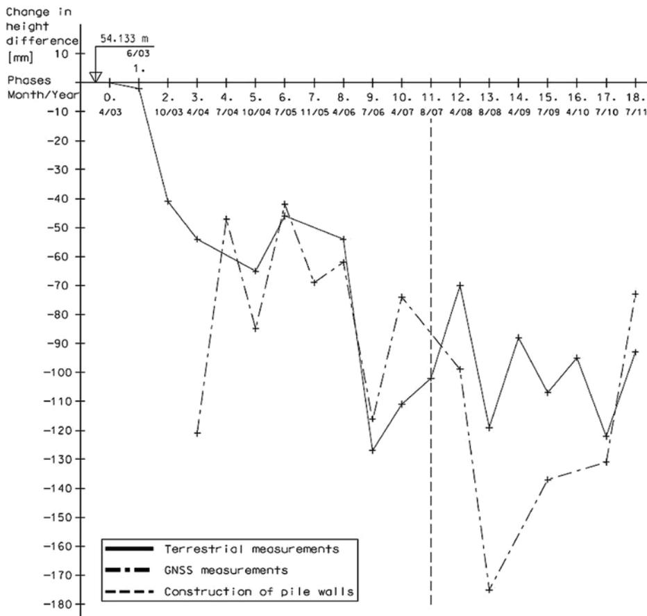
**Fig. 11** Changes in height difference between Rab03–Rab02 points.
