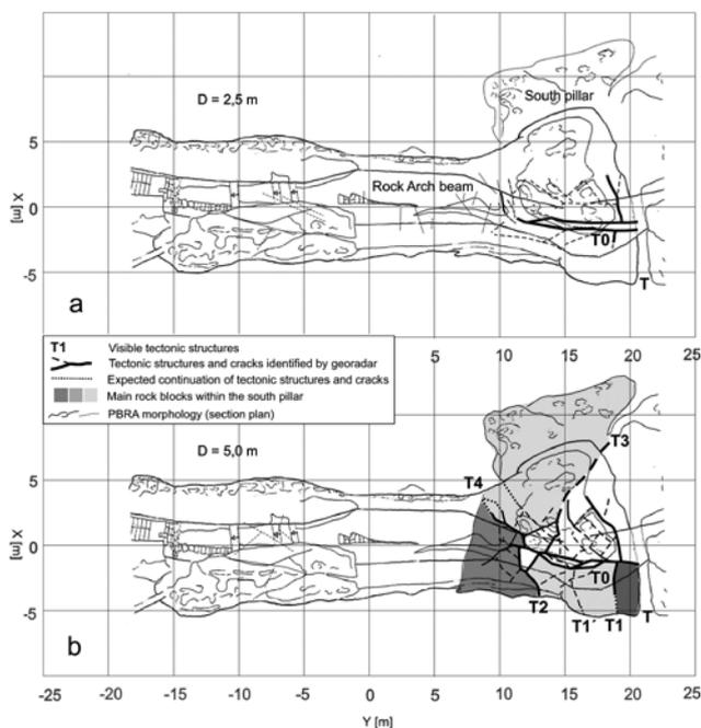
**Fig. 4** Areal correlation of the course of the joint system in horizontal (ground plan) cross-sections in two depth levels from the cross-beam surface (2.5 metres/A – 5.0 metres/B) with the introduced visualization of real joints and with an indication of the main rock blocks of the pillar at the level of the horizontally trending layer.
