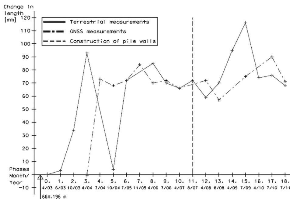
Fig. 8 Changes in length between Rab03–Rab02 points. Source: Rytíř 2012, Riegerová 2012
