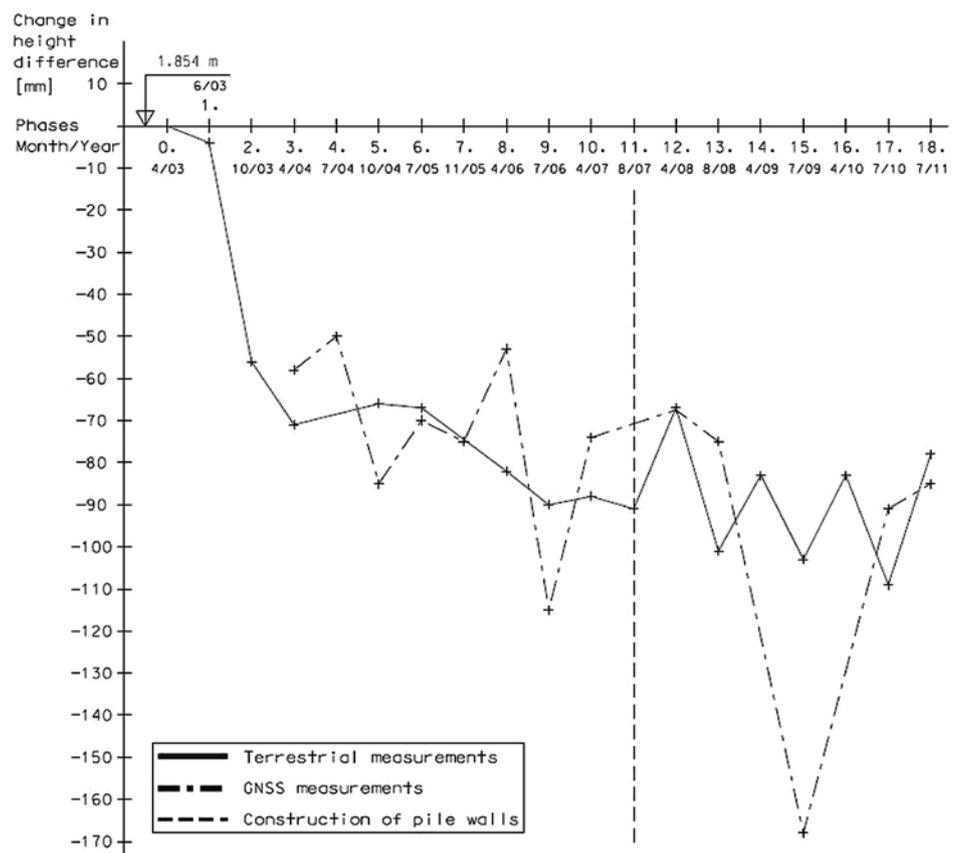
**Fig. 10** Changes in height difference between Rab01–Rab03 points.
