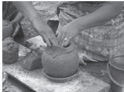
Figure 18. Rolling process, modeling the neck of a pitcher, Yoncultac village, Huehuetenango, Guatemala. Photo: Julio Hernández.
