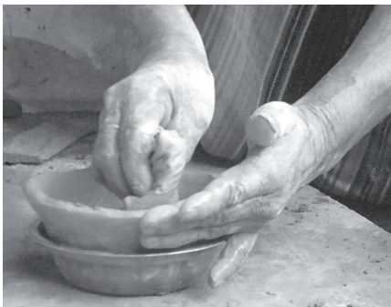
Figure 23. Smoothing process, using a piece of cloth, San Mateo Ixtatán, Huehuetenango, Guatemala. Photo: Julio Hernández.
